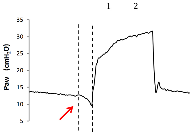
Figure 1: Negative deflection of the pressure wave due to the patient's inspiratory effort (red arrow). The two dotted lines indicate the beginning of the patient's inspiratory effort (1) and the delayed ventilator support (inspiratory delay) (2).
