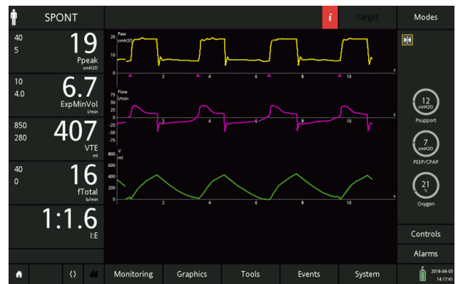
Figure 9: The same patient ventilated with inspiratory trigger sensitivity: 2 l/min, expiratory trigger sensitivity: 25%, ramp: 75 ms (top), immediately after changing the ETS to 10% (middle; red line), and after a few breaths with ETS at 10% (bottom). Note the prolonged inspiration with evident late cycling in the first breath after the settings have been changed (red arrow), and the effect on the triggering phase soon leading to ineffective efforts (white arrows).
